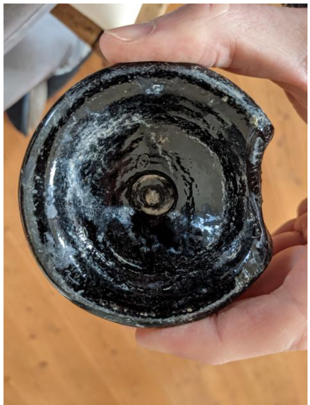
Base of small-diameter bottle 307:16 showing rod or tool mark at base in centre
