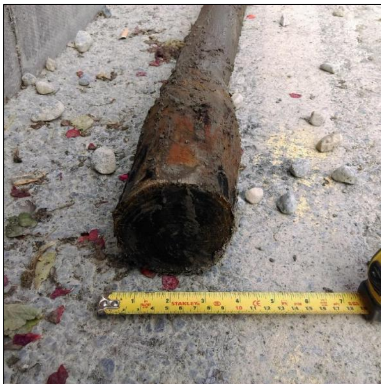
Pl. 10 Wooden stopper or plug at base of pump mechanism.
